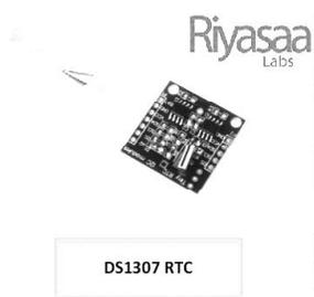
*Realtime Clock (RTC) module can saves the current time – even if the power supply is not present – due to the small battery. On computer mainboards such a module is installed, which is why the time of the computer does not have to be re-adjusted every time you restart. Since the Raspberry Pi / Arduino does not carry an RTC module from within, this can be retrofitted*
