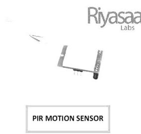
*The PIR motion sensor has some advantages over other similar products: besides the low price, a signal is sent only if something moves. This allows you to wait for signal flanks using the GPIOs. In addition, a resistance can be varied so that a signal is only sent when the movement is close, or changes that are already far away are perceived.*
