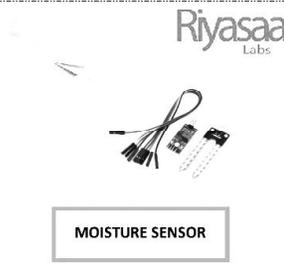
*This analogue humidity sensor finds an excellent place in automatic irrigation systems. It is placed in the ground and measures the humidity by current flowing between the strands. The more humid the earth in between, the higher the (analog) signal. In order to read the value with the Raspberry Pi, the [MCP3002](#) is needed (Arduinos can recognize analog signals directly).*
