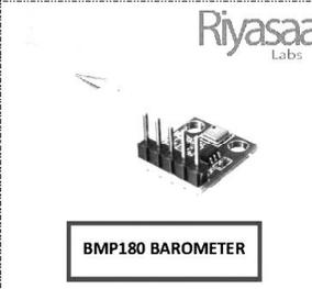
*The determination of the air pressure can be meaningful in weather stations and similar projects. This is best done using the BMP180, which is controlled via I2C on the Raspberry Pi. In addition to the air pressure, the temperature can be read out as well as the altitude.*
