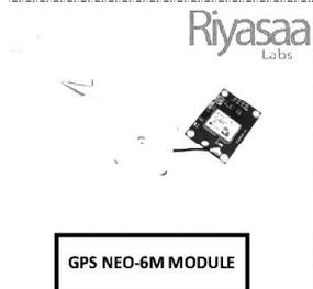
*The most common and best known GPS receiver is the NEO-6M module. All GPS position data can be determined with the help of the orbiting satellites. In addition, it is compatible with the Raspberry Pi packages minicom and gpsd, which makes reading the coordinates very easy.*
